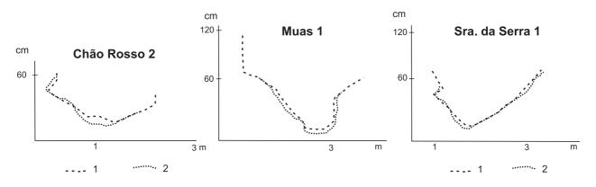
FIGURE 1. Longitudinal profile and evolution of gullies studied in Serra do Marão (Pedrosa, 1993). Line nr. 1 represents the starting stage and line nr. 2 its evolution.
